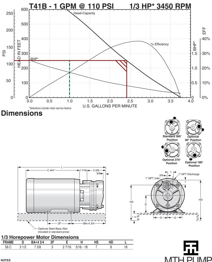
All dimensions in inches. May vary ± ¼ inches. Not for construction purposes unless certified. \*See motor dimensions for "C-AH" dimension (Varies depending on motor enclosure).
